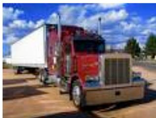
semitrailer is legally defined as a vehicle designed so that a portion of its weight rests on a towing vehicle. This distinguishes it from a full trailer on which the entire load, except for a drawbar, rests on its own wheels.”
